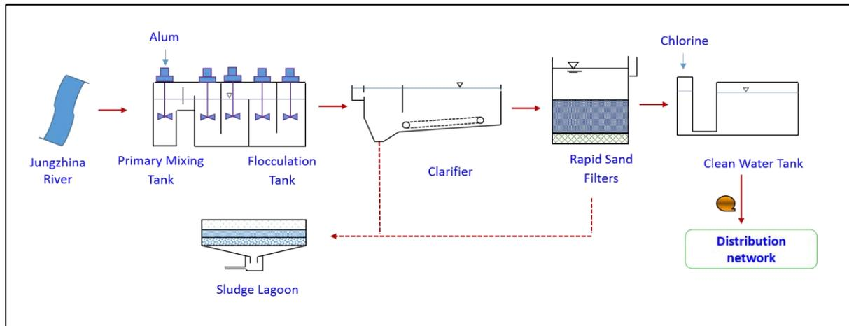
**Figure 2: Schematic Diagram of Water Treatment Processes**
