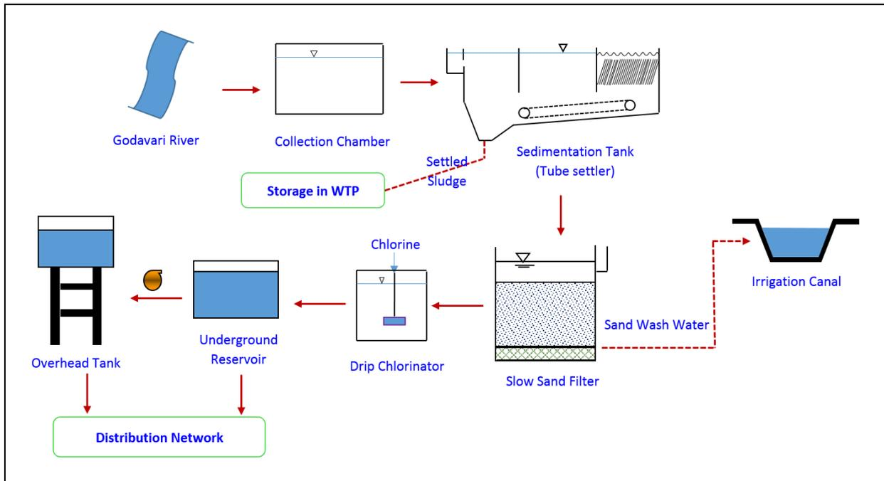
**Figure 1: Schematic Diagram of Water Treatment Processes**
