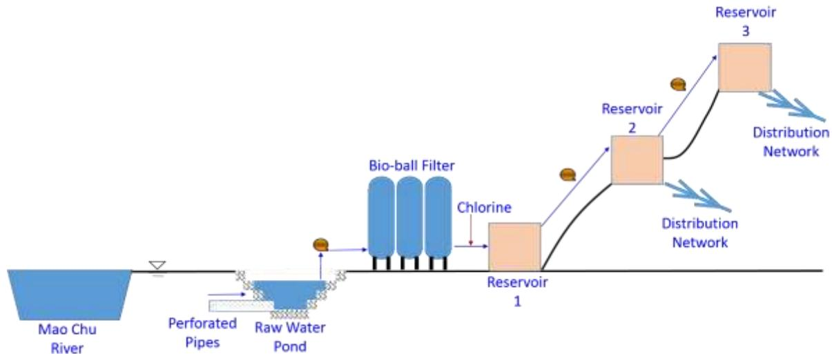
**Fig 2: Schematic Diagram of Water treatment process**
