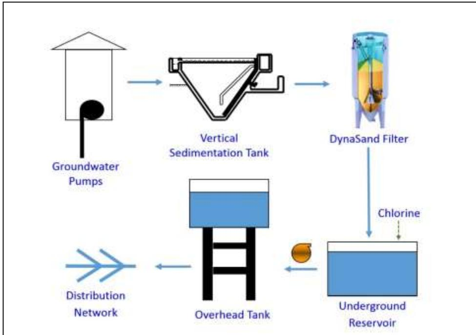
**Figure 1 Schematic Diagram of Water Treatment Processes**
