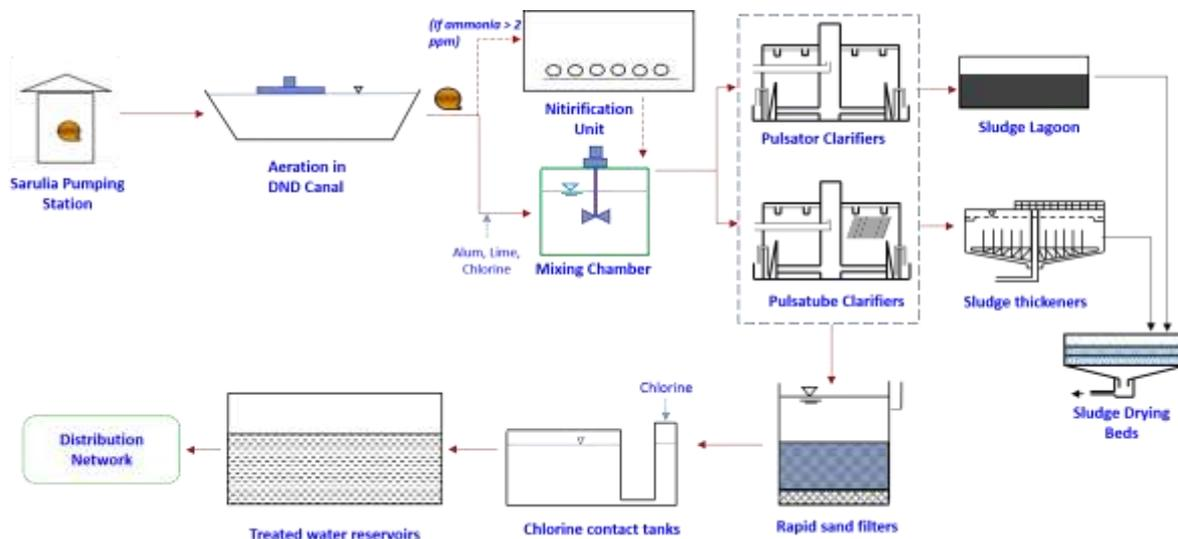
**Figure 1: Schematic Diagram of Water Treatment Processes**
