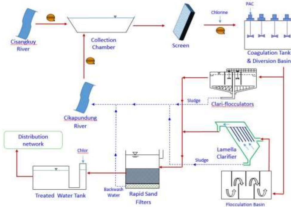
**Figure 3 Schematic Diagram of Water Treatment Processes**
