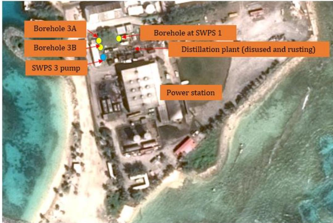
*Figure 4: Southern Ebeye location showing locations of water supply infrastructures (GHD, 2014)*
