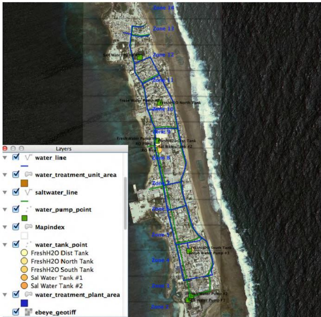
Figure 2: Overview of Ebeye Water Supply System (GHD, 2014)
