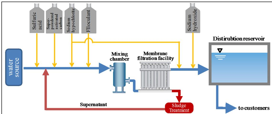
Figure 3 | Ceramic membrane facility at Kawai
