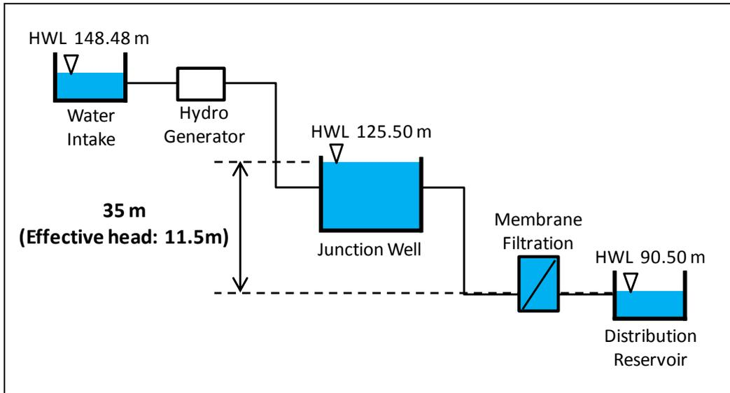
Figure 2 | Use of natural energy for membrane filtration
