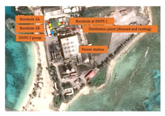
Figure 4: Southern Ebeye location showing locations of water supply infrastructures (GHD, 2014)
