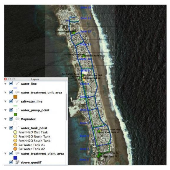
Figure 2: Overview of Ebeye Water Supply System (GHD, 2014)
