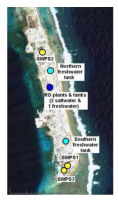
Figure 3: Seawater pump station locations (GHD, 2014)
